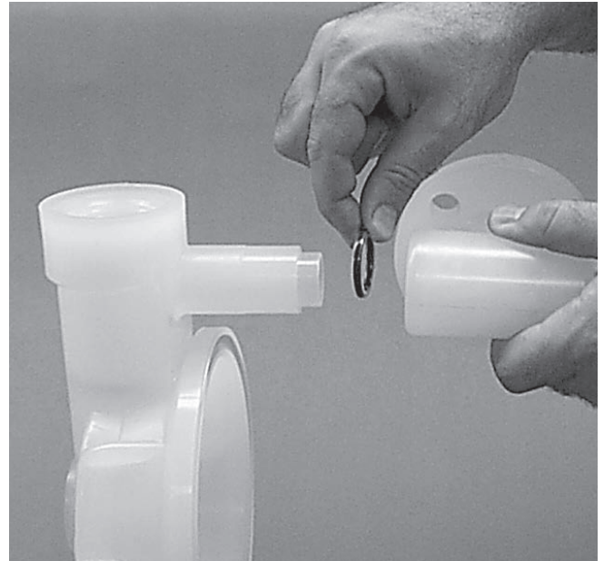
Step 10. Figure 10 Remove tee section from liquid chamber and inspect o-rings for signs of wear. Replace worn parts with genuine Wilden parts for reliable performance.
