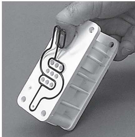
Step 3. Figure 3 Lift away air valve assembly and remove air valve gasket for inspection. Replace if necessary.
