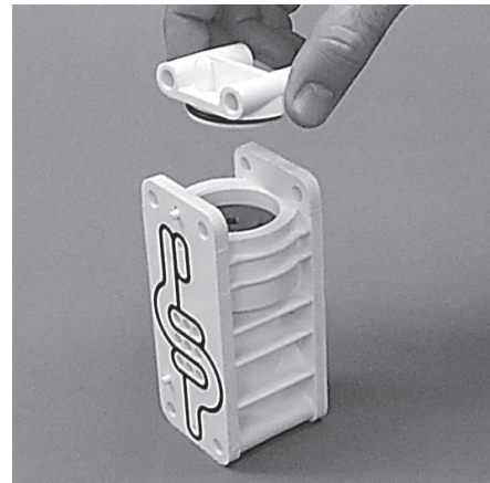
Step 4. Figure 4 Remove air valve end cap to expose air valve spool by simply lifting up on end cap once air valve bolts are removed.
