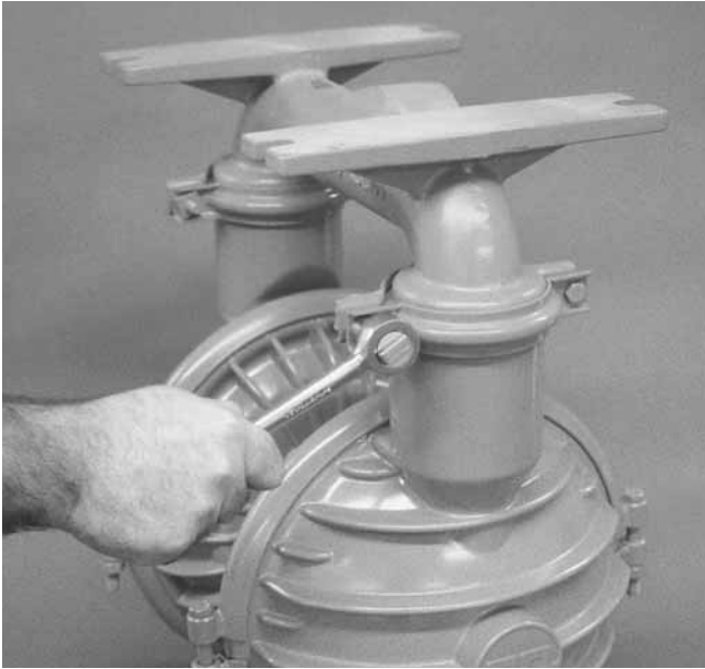
Step 4. Figure 4 Remove the two small clamp bands that fasten the intake manifold to the liquid chambers.
