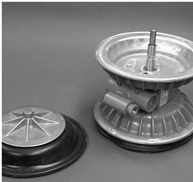
Step 9B. Figure 9B 2) The outer piston, diaphragm, and inner piston separate from the shaft which remains connected to the opposite side diaphragm assembly. Repeat disassembly instructions for opposite liquid chamber. Inspect diaphragm assembly and shaft for signs of wear or chemical attack. Replace all worn parts with genuine Wilden parts for reliable performance.
