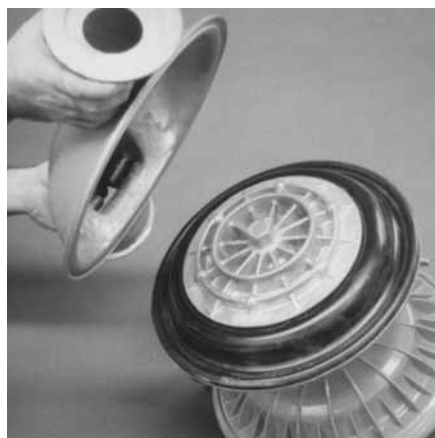
Step 7. Figure 7 Lift liquid chamber away from center section to expose diaphragm and outer piston.
