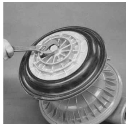
Step 8. Figure 8 Using an adjustable wrench, or by rotating the diaphragm by hand, remove the diaphragm assembly.
