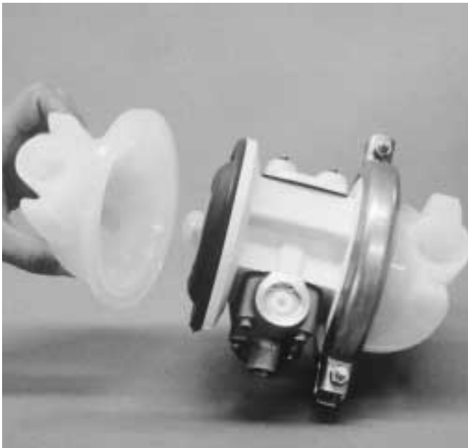
Step 9 Figure 9 Lift the liquid chamber away from the center section to expose the diaphragm and outer piston. ( Figure 9 )
