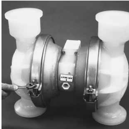
Step 9. Figure 9 Remove one set of large clamp bands which secure one liquid chamber to the center section.
