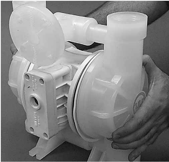
Step 9. Figure 9 After clamp bands are removed, pull liquid chambers apart.
