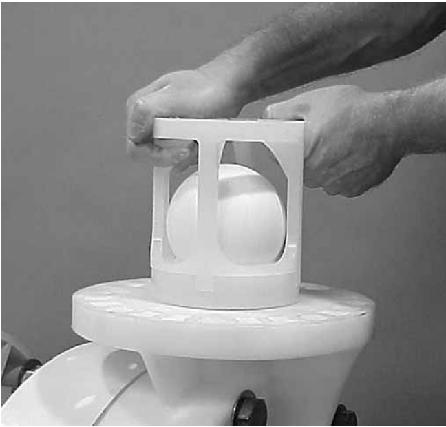
Step 4. Figure 4 Rotate the ball cage counterclockwise to remove the threaded ball seat. The ball cage has feet that interlock with the seat to facilitate this operation.
