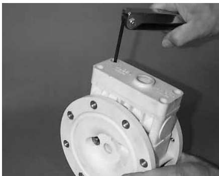
Step 1. Figure 1 Loosen the air valve bolts utilizing a 3/16" Allen wrench.
