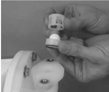
Step 3. Figure 3 Remove the discharge manifold to expose the valve balls, valve seats and valve seat o-rings.
