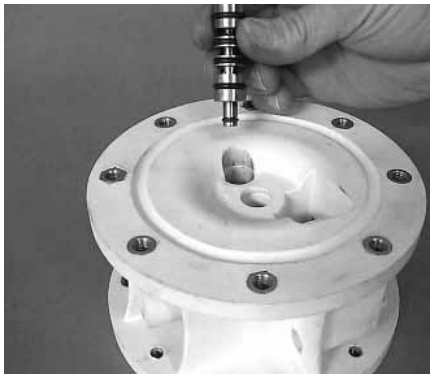
Step 7. Figure 7 Remove pilot spool sleeve from center section.
