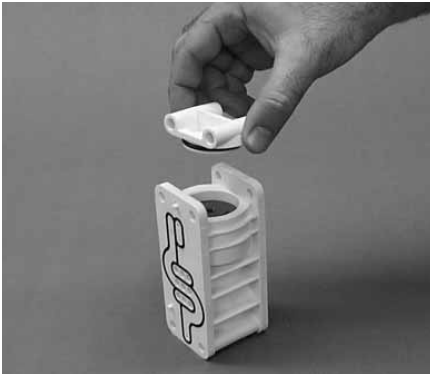
Step 4. Figure 4 Remove air valve end cap to expose air valve spool by simply lifting up on end cap once air valve bolts are removed.
