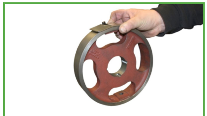
Figure 9 Mounting rotor shims on the rotor (Step 1)
