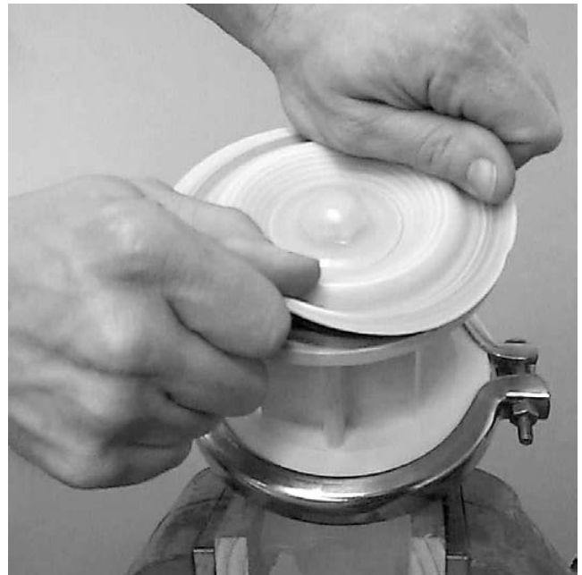
Step 11. Figure 11 Using an adjustable wrench, or by rotating the diaphragm by hand, remove the diaphragm assembly from the center section. (Figure 11)
