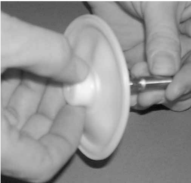
Step 10. Figure 10 For PTFE fitted pumps diaphragms, remove diaphragm by turning in a counter-clockwise direction.
