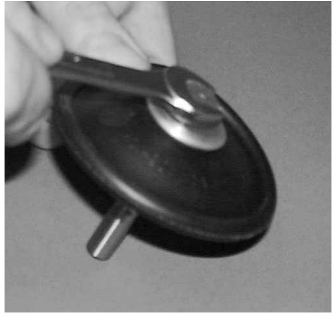
Step 9. Figure 9 Remove shaft and attached outer piston from the center section. Hold the diaphragm and remove outer piston with 7/16" wrench. If unable to remove diaphragm, place shaft in a vise equipped with soft jaws. NOTE: See Step 10 for PTFE fitted pumps.
